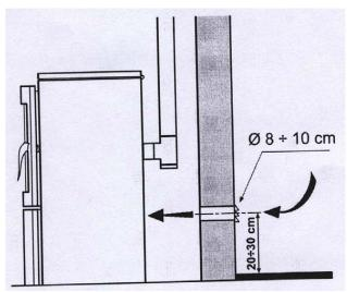
Figure 8.Minimum distances for the installation of the ventilation grid
